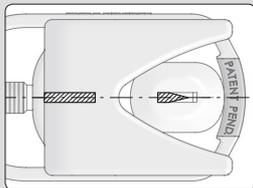
**Note** *Some knives are difficult to mount in line with the Guide Bar. Knives can also be sharpened with asymmetrical bevels. In these cases, and if the angle is not correct when you turn over to sharpen the second side, you can adjust it separately with the Micro Adjust.*
