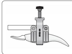
The shape of the knife handle determines how far into the holder the knife needs to be mounted. Make sure it is secured.
