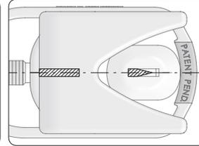
Check that the knife blade is in line with the Guide Bar.
