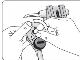
Mount the Guide Bar in the jig with the small adjustment screw.
