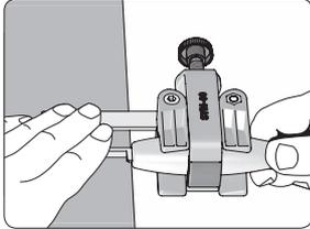
Mount the knife in the holder whilst lying flat on a table edge.
