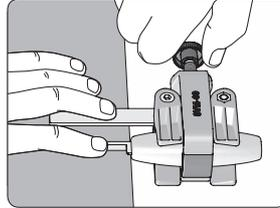
Press the Guide Bar and the knife blade against the table. Lock the knife with the Knob.
