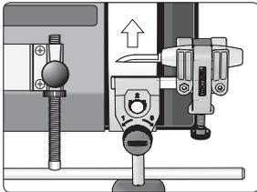
You can also sharpen away from the edge with the Universal Support mounted horizontally. If your machine is placed on a bench over 700 mm high (27½") this will give a better working position. Some prefer this position since the knife cannot cut into the grinding wheel. It can also be advantageous if for some knives you want to have a slower grind.
