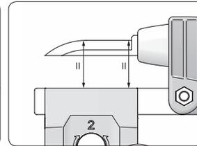
Check that the knife edge is parallel to the SVM-45. Tighten the large black knob.
