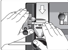
The Universal Support is normally mounted vertically for sharpening *towards* the edge. It will give you a more effective grind and you will get less burr to remove when honing. For folding knives (which cannot be locked) you should work in this position to prevent the knife blade from closing during the sharpening.
