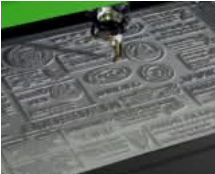
Engraving & laser cutting of custom ink stamps
