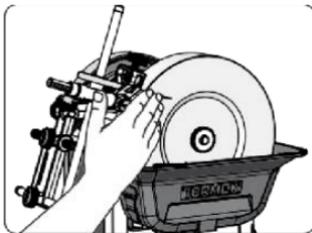
Adjust the sharpening pressure with a finger and check what sharpening is carried out. Fine adjust if necessary.
