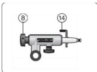
Mount the screw (8). Lock the shaft with the Allen key (14) when tightening.
